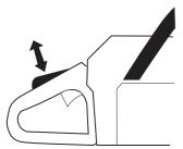
• Check that the throttle control and throttle lockout move freely and that the return springs work properly.
